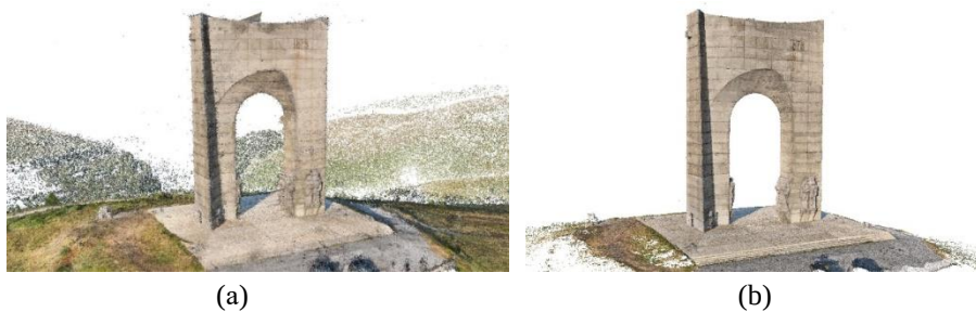
Fig. 4. Comparison of the generated point cloud before and after applying filtering
